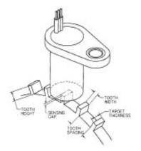
Speed or RPM sensing can be used for a variety of applications including: camshaft and crankshaft, transmission, tachometers, antiskid/traction control, sprocket speed, conveyor speed, stop motion detection, counters. Speed sensing is done in applications in: automotive, agricultural and construction equipment, buses, trucks, lawn and garden equipment, golf carts, ski mobiles, escalators, and automation equipment to name a few.
